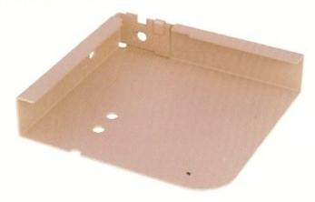
The standard shelf is double folded with closed corners and has a two way locking mecanism at each corner. Made from 18 gauge steel. Standard sizes include 12", 15", 16", 18", 24", 30", 32", and 36" deep, by 36", 42", and 48" wide.
